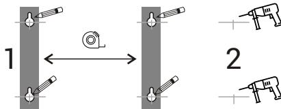
Insert the dowels in obtained holes and screw in quick mounting screws, leaving 5 mm to the wall.
